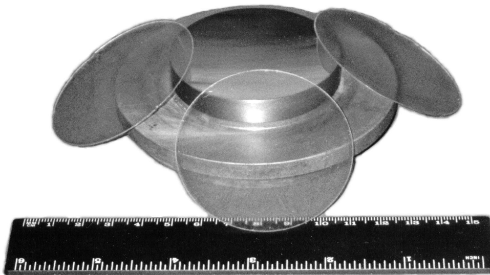
Fig. 3. Thin CsI(Tl) slices made by plastical deformation.
